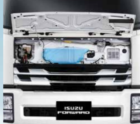
▼ Quick access panel. Designed for convenience, inspecting or replacing clutch fluid, wiper fluid and cabin air filter can be done quickly and safely.
