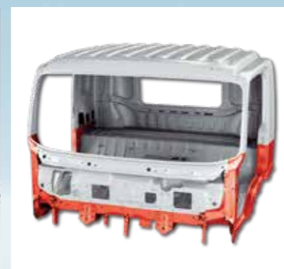
▲ High rigidity cab with cation electrodepositing coating.
