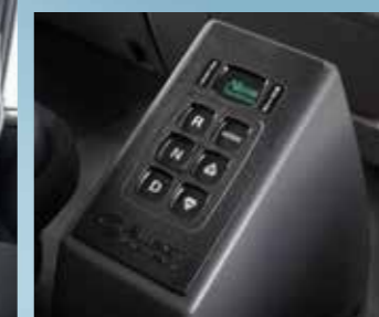
▲ Allison electronic control with digital display.
