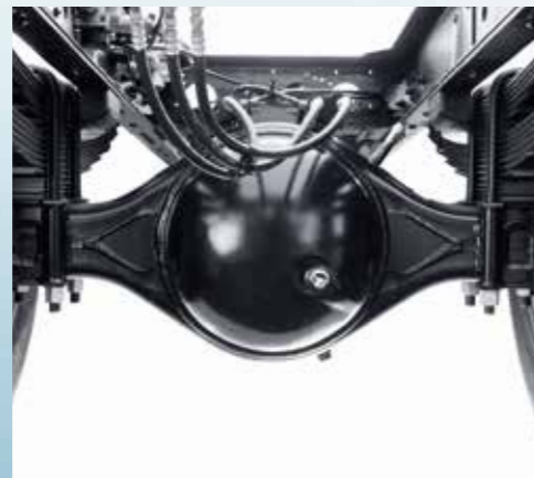
▲ Bigger rear axle capacity (13 ton).
