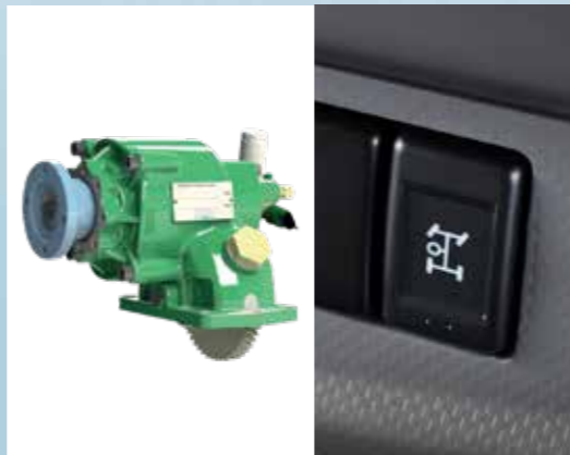
▲ Hot Shift PTO with external speed controller and safety features.
