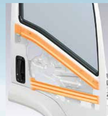
▲ Door impact beam with high tensile strength reinforcement frame.
