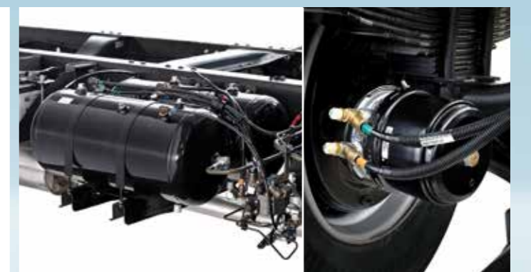
▲ Full air brakes with auto adjuster.
